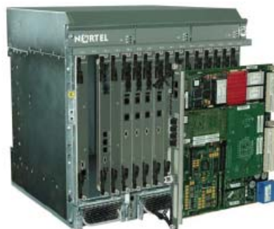
Nortel's ATCA-compliant VSE-based MSC Server
